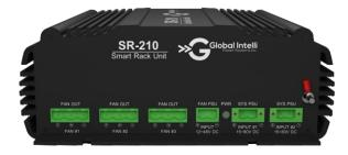
The SR-210 is energy efficient as it not only assists in conserving power by selectively switching off the rack's cooling fans according to the prevailing temperature conditions in the equipment rack but also greatly increases the life span (MTBF) of the fans, as the fans are switched off when they are not required to operate, while always maintaining the user defined ambient temperature.
